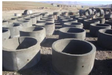
Fig 12 – Well rings at the manufacturing yard
